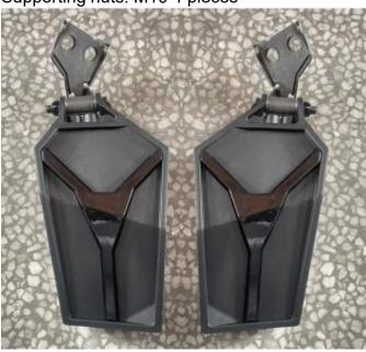
2. First, unscrew the screws at the A-pillar of the original vehicle and replace them with the screws that match the product. Then, install the side mirror on the screws and use the matching nuts to fix it. Finally, adjust the angle of the side mirror to the appropriate angle. (The other side mirror is installed in the same way). As shown below:
