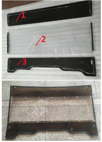
3. Use 2pcs M6\*20 screws, 2pcs M6 flat pads, 2pcs M6 nuts and 2pcs M6\*10 outer hex screws with pads to fix the windshield on the front frame with two iron brackets. As shown in the figure:
