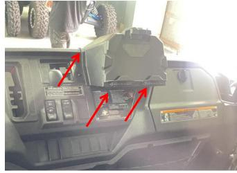
4. Cut the sponge strip from the kit to a proper length and attach it to the device holder. As the picture shows:
