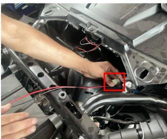
3. Pull the remaining adapter wire along the vehicle gap to the front grille, and connect it with the harness of the fang lights on the grille. Then start the vehicle to check whether the fang lights light up normally, and install the grille back to its original position after confirmation. As shown in picture:
