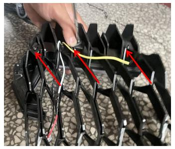
2. Next, remove the hood of the original vehicle, open the mudguard inside the hood, locate the wire harness plug-in reserved for the original vehicle, and connect the adapter wire in the accessory package to the original vehicle plug-in. As shown in picture:
