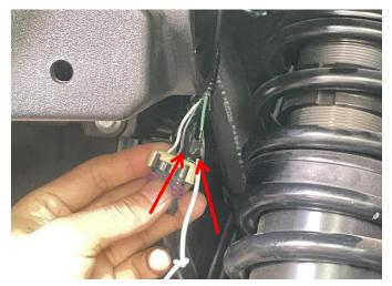
4. Pull the extension cable that has been connected to the power supply along the gap to the grille and connect it with the grille light. Then, install the grille and prepare a 6.5mm drill bit. Drill corresponding screw holes according to the screw hole positions on the grille. Then, attach a steel card to the hole position and fix it with screws.As shown in picture:
