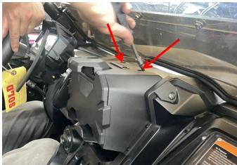
3. Finally, cut the sponge strip from the accessory package to a suitable length and stick it onto the electronic device holder.As shown in picture:
