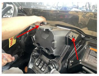
2. Press the positioning hole at the edge of the electronic device holder, and use the matching Self-tapping screw to fix it in turn.As shown in picture:
