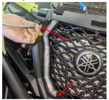
3. Open the cover of the original vehicle, find the wiring harness plug-in of the original vehicle daily running light and disconnect it. Then prepare the conversion cable for the fang light, connect it with the original vehicle daily running light and the vehicle wiring harness plug-in, and then pull the conversion cable to the grille, connect the fang light respectively, and finally install the cover.As shown in picture:
