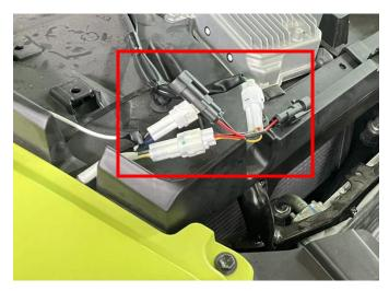
5. Thread the wire harness of the decorative lights on both sides through the gap to the adapter line, and connect it with the plug-in on the adapter line. Then start the vehicle to turn
