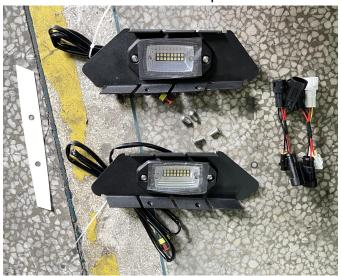
2. First, remove the plastic front fascia from the original vehicle, take out the positioning paper from the accessory package and place it on the front fascia. Use a 6MM drill bit to position and drill out screw holes on the paper. (The positioning paper is not divided into left and right sides and can be used in both directions). As shown in picture:
