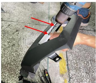
3. Install the decorative light on the front fascia and secure it with matching screws (the reinforcing ribs on the back of the front fascia need to be correspondingly stuck in the slots on the edge of the decorative light rear shell). As shown in picture:
