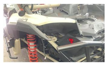
4. After removing the original tail light from the mounting frame, replace it with a new one.
