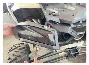
5. After reconnecting the tail light harness plug-in, then reinstall the tail light frame back into the original vehicle, and finally screw back the previously removed screws. (The other side is installed in the same way as above)
