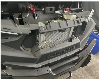
2. Install the new headlights according to the fixing method of the original headlights, then connect the plug-ins of the headlights with the wiring harness of vehicle, and finally install back the decorative panels and the engine cover. As the picture shows:
