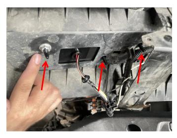
2. Connect the plug-in of the wiring harness on the new taillight to the integral wiring harness plug-in, and then install back the rear bar in place. As the picture shows:
