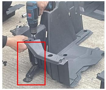
3. Load the rear cargo box with the iron bracket onto the vehicle and use the screws of the original vehicle to fix it. The splicing place in the cargo box is directly fixed with the ball head screw of the original vehicle. Finally, the
