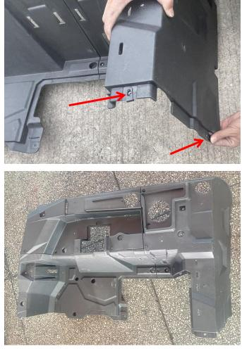
2. Remove the rear seat, C-pillar frame and spare tire support of the original vehicle, then remove the rear cargo box on the left side, and move the iron bracket on the original cargo box to the new cargo box according to the original position. As the picture shows:
