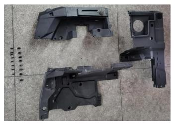
1. Assemble all the parts together, take out the steel clips from the accessories package and clamp the steel clips in the limit slots of the splicing edge, and then fix with screws. As the picture shows:
