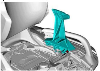
tightening torque Hex. Scotch Grip Screw M10 X 50 [P7] 29 ± 3.0 N•m (21 ± 2 lbf•ft)
