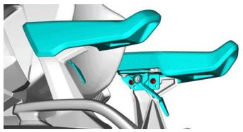
tightening torque M6 X 16 Torx Screw [P8] 8 ± 1.0 N•m (71 ± 9 lbf•in)
