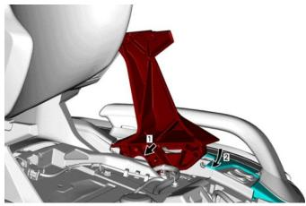
Step 1: Install armrest support on tube Step 2: Rotate to align the front holes
