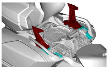
3. Secure with M10 X 50 hex. scotch grip screw [P7] and flap gasket [P9] and tighten to specification.
