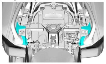
tightening torque Access cover retaining screw 29 ± 3.0 N•m (21 ± 2 lbf•ft)
