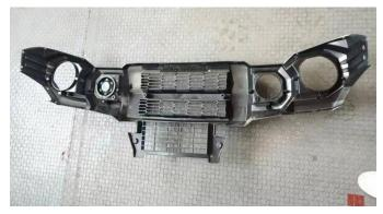
2. Move all the steel clips and accessories from the original headlight onto the new headlight, and then fix the new headlight on the bumper. As shown in picture:
