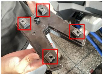
3. Connect the new taillight to the original vehicle taillight harness, and finally secure it with the original vehicle screws. (Install the tail light on the other side in the same way).As shown in picture:
