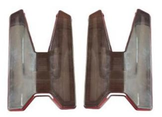
2. First, remove the original vehicle's taillights and move the steel clips on the rear housing of the original taillights onto the new taillights.As shown in picture:
