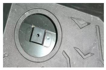
2. Use scissors to cut out the template paper, corresponding to the left and right holes, mark with a marker, and then use a utility knife to cut out the gap. As shown in picture:
