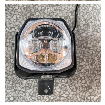
3. Install the new headlights back onto the original vehicle, connect the wiring harness connectors, and finally reinstall the hood.
