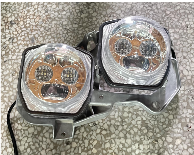
3. Reinstall the bracket of the installed lamp back into the original vehicle, connect the wiring harness plug of the headlight, and finally reinstall the hood. As shown in picture:
