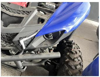
2. After removing the original headlight from the installation shell, replace it with a new headlight. (It can be fixed using the original vehicle screws or the product's matching screws).As shown in picture:
