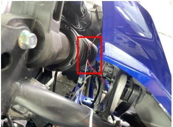
4. Select any point on the extension line to remove its outer skin, then prepare a new extension line and connect it to it. Connect the remaining end to the red light guide wire on the other side of the headlight, and provide insulation protection. Finally, reinstall the previously disassembled accessories. The exposed extension cable can be hidden under some decorative pieces. As shown in picture:
