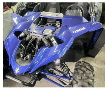
2. Remove the mounting bracket of the original headlight and disconnect the wiring harness connector. Then, remove the original headlight from the mounting bracket and fix the new headlight on the mounting bracket using the original method (it can be fixed using the original vehicle screws or the product matching screws). Install the other headlight in the same way as above. As shown in picture:
