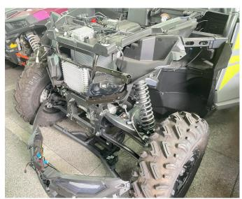
2. Remove the original daytime running light from the front fascia and replace it with a new one, using the original vehicle screws for fixation. (The daytime running lights on the other side can be replaced and installed in the same way.). As shown in picture:
