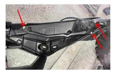
3. Reinstall the front fascia of the replaced daytime running light back into the original vehicle, and connect the wiring harness plug of the daytime running light. Then, start the vehicle to check whether the daytime running light is on normally. Once confirmed to be correct, the previously removed hood and decorative panel can be reinstalled. As shown in picture:
