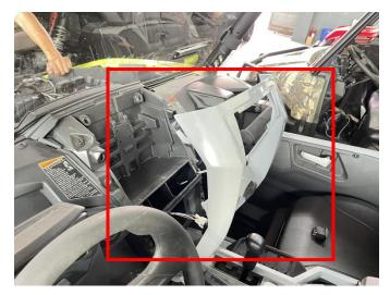
2. Open the cover of the original vehicle, thread the control switch wiring harness on the hood scoop light through the cable outlet hole in the cabin to the center console of the cab, and then move to the cab, connect the control switch matching the product with the wire harness according to the installation sequence on the picture, and then put the control card on the control panel. If the rocker switch cannot be inserted properly, a blade can be used to
