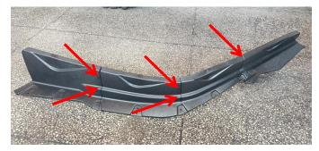
5. Refer to step 3 to place the fender flares in the original vehicle installation position, and then prepare a 6mm drill bit to drill fixing holes in sequence according to the screw holes on the wheel arch, and fix it with matching screws and nuts. As shown below:
