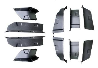
1. First, assemble the split front fender flares into a whole with screws.As shown in picture:
