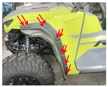
Installation steps for rear fender flares:4. Install the small fender flares below the rear
