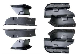
1. First, assemble the split front fender flares into a whole with screws.As shown in picture:
