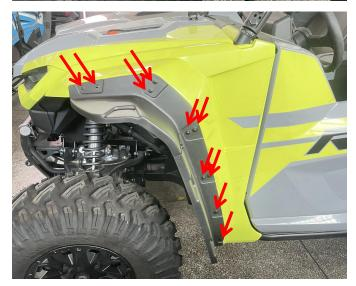
Installation steps for rear fender flares: 4. Install according to the installation method of the front fender flares. (Install the other side in the same way).As shown in picture:
