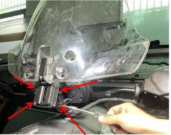
3. The height of the windshield can be adjusted by the trigger on the windshield.
