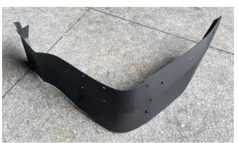
2. Install the assembled fender flares onto the original vehicle fender flares, and use 6MM and 8mm drill bits to drill fixing holes according to the positioning holes on the added fender flares. Then, use screws and nylon buckles for fixation. As shown below:
