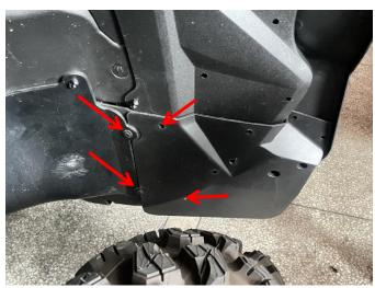
4. Using an 8mm drill bit, punch the hole positions in sequence according to the positioning holes on the mudguard, then use a snap fastener to fix them, and use screws and nuts to fix the remaining screw holes. As shown below:
