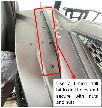
7. Take out the iron bracket that comes with the product and fix one end of the bracket to the wheel arch and the other end to the original rear cargo box of the vehicle. As shown below: Note: It is necessary to drill a fixing hole with a 6mm drill bit in advance based on the position of the iron bracket on the rear cargo box, and then use screws and nuts for fixation.
