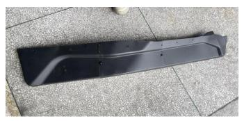
6. Install the assembled rear fender flares onto the original fender flares, and use 6MM and 8mm drill bits to drill fixing holes according to the positioning holes on the added fender flares. Then, use screws and nylon buckles for fixation. As shown below:
