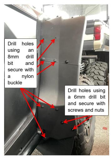
3. Finally, install the mudguard on the fender flares. First, pry out the snap fastener on the original vehicle mudguard, and then install the upper mudguard before reinstalling the snap fasteners. As shown below:
