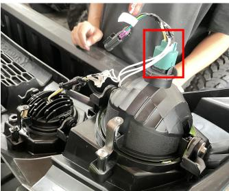
5. Install the grille with the installed headlights back into the original vehicle and fix it. Finally, connect the remaining plug on the adapter line with the wiring harness plug of the entire vehicle. As shown in picture:
