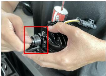
3. Use the longest screw in the accessory package, pass through the iron bracket and spring, and use a square screw to fix the iron bracket to the headlight (the height angle of the headlight can be adjusted through this screw). After completion, the headlight can be fixed on the original grille. As shown in picture:
