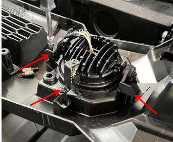
4. Connect one end of the matching adapter cable for the headlight to the new headlight harness connector, and the other end to the original headlight. (The other headlight is assembled and fixed in the same way). As shown in picture:
