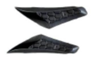
2. Place the rear wheel well block off at the air inlet of the rear door and secure it with the self tapping screws provided with the product. (Installed in the same way on the other side).As shown below:
