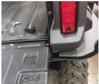
3. Install the new bracket on the rear gate with the screws and nuts just removed, and the installation is complete, as shown in the figure.
