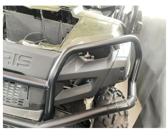
2. Connect the conversion cable of the headlight to the new headlight wiring harness, and then install the new headlight to the original vehicle, and fix it with the original screws. As the picture shows:
