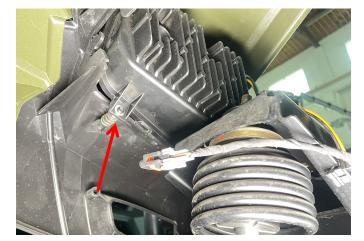
3. Finally, connect the other end of the conversion cable plug-in with the original vehicle wiring harness plug-in, and then reinstall the original vehicle cover. (The headlight on the other side shall be replaced and installed in the same way as above). As the picture shows:
