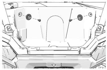
3. Insert two screws and attach cargo box to vehicle. Torque screws to specifications.
