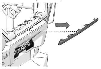
5. Insert center accent light (3) to vehicle with four hex nuts. Torque nuts to required specification.
