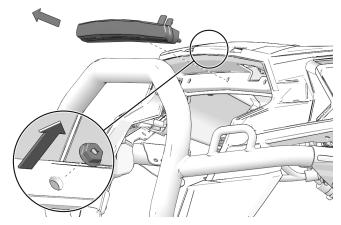
2. Attach front accent light assembly(1) with three hex nuts(2). Torque nuts to required specification.
