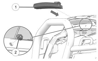
3. Remove socket cap and connect power cable to front access light assembly.
