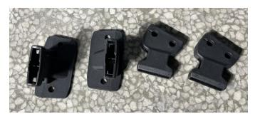
1. Remove the front door buckle support of the original vehicle, replace it with a new support, and then fix it with the original vehicle screws. (The other side is installed in the same way). As the picture shows:
