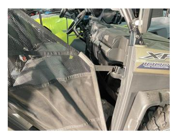
2. Remove the rear door buckle support in the same way as above, replace it with a new support, and then fix it with the original screws and nuts. (The other side is installed in the same way). As the picture shows:
