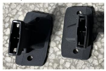
1. Remove the front door buckle support of the original vehicle, replace it with a new support, and then fix it with the original vehicle screws. (The other side is installed in the same way). As the picture shows:
