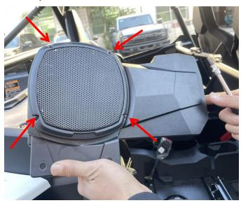
2. Remove the rear seat of the original vehicle for subsequent installation. Then unscrew the screws on the original vehicle, connect the audio with the wiring harness plug-in of original vehicle, use the screws of original vehicle to fix
