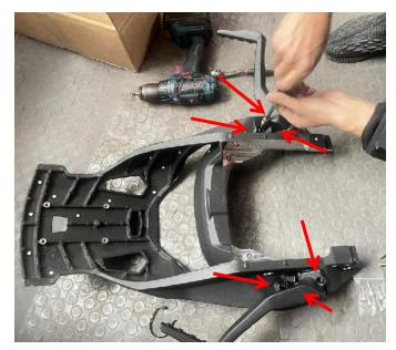
5. Place the product's connecting block under the vehicle's seat cushion, and then install the seat mounting bracket back into the vehicle.
