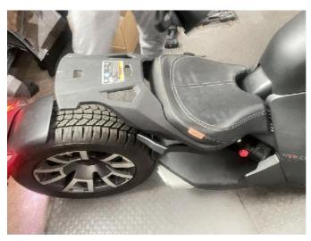
6. Use the M6\*20 screws in the kit to fix the connecting block just placed with the seat mounting bracket, and then screw back the original screws that were removed before.
