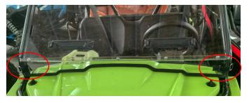
4. Then, secure the windshield to the front roll bar with four large straps. As the picture shows:
