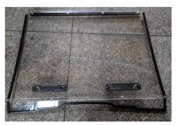
3. Using two small straps to secure the windshield to the lower end of the front roll bar. As the picture shows:
