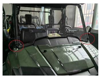
3. Then, secure the windshield to the front roll bar with four large straps.
