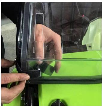
3. Then, secure the windshield to the front roll bar with two large straps.
