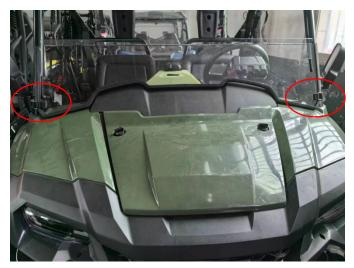
3. Then, secure the windshield to the front roll bar with two large straps.
