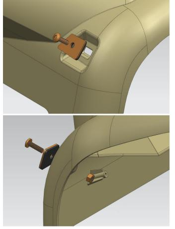
9. Finally, fix the 4 hook shaped installation brackets that come with the product on both sides of the roof (2 on each side and fixed with self tapping screws)As shown below:
