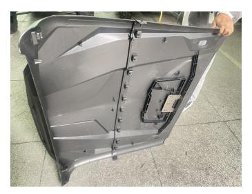
6. Place the assembled roof onto the original vehicle, align the screw holes on the iron plate bracket with the screw holes on the original vehicle frame, and fix them with M6\*16 screws.As shown below:
