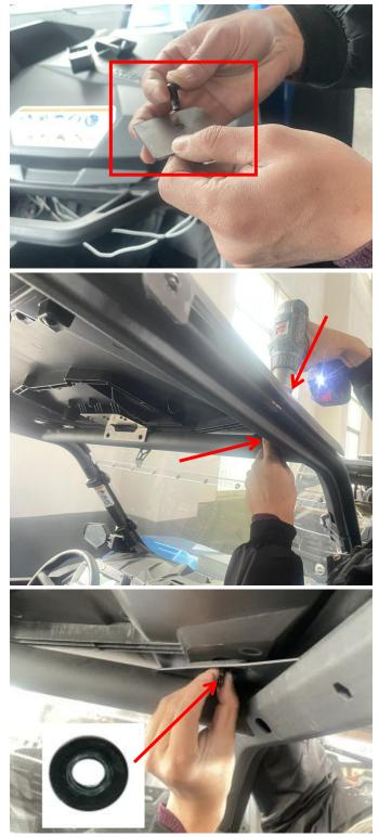
8. When fixing the rear ends of the roof, it is necessary to use M6\*35 screws, put on square gaskets, paste sponge pads on the back, and fix with nut flat pads.As shown below:
