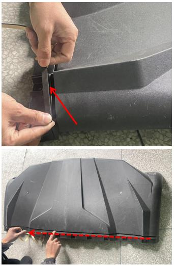
3. After the sponge pad is affixed, use the self-tapping screws (each screw needs to add a flat pad with an outer diameter of 14mm) to assemble the separate roof into a whole.As shown below:
