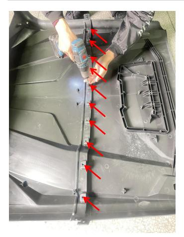
4. Insert steel clips at the beginning and end of the intersection of the two roofs (onto the roof with sponge pads) and secure them with M6\*16 screws.As shown below:
