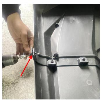
5. Use M4\*14 self tapping screws from the accessory package to secure the "L" shaped iron plate bracket to the roof.As shown below:
