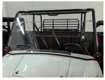
4. Then, secure the windshield to the front roll bar with two large straps and two small straps. As the picture shows:
