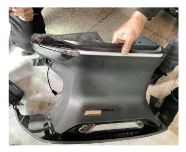
6. After the product installation is completed, one end of the supporting adapter cable is connected to the plug-in reserved for the vehicle, and the other end is connected to the wiring harness plug-in of the product, after which the vehicle is started to see if the light are normally lit, and then assemble the parts after confirming that it is correct.
