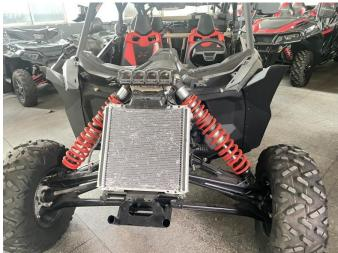
5. Remove the center mesh, headlights and daytime running lights connected to the original front fascia cover, then replace the original cover and reinstall the new front fascia cover (the original cover has 2 through-hole rubber plugs, which need to be pried down and installed on the original cover), and then install the previously removed headlights, center mesh and other accessories back to the original position after the replacement is completed.
