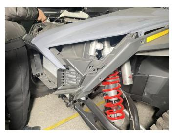
2. Move the "H" shaped rubber stopper and plug on the original headlight to the new headlight according to the original positions, and then install the new headlight back to the original vehicle, connect the wiring harness plug-ins and start the vehicle, open the switch of headlight, check whether the new headlight work normally, and then use the screws and springs of original vehicle to fix it. As the picture shows:
