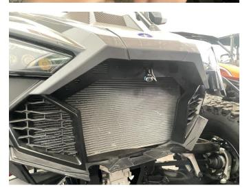
2. Install the new day running light on the vehicle, connect the wiring harness plug-in, and use the original thread sleeves to fix it, then install the original mesh grill back. As the picture shows:
