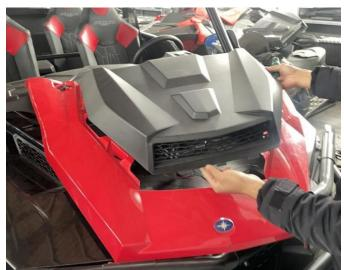
2. When installing the new hood, the limit brackets on the hood need to be correspondingly inserted into the slots on the decorative panel of the original vehicle, and then fix the hood with the original screws. As the picture shows:
