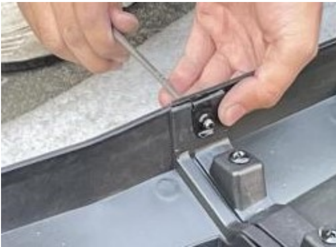
2. Fix the two iron square mounting brackets in the package to the roof with self-tapping screws. As the picture shows:
