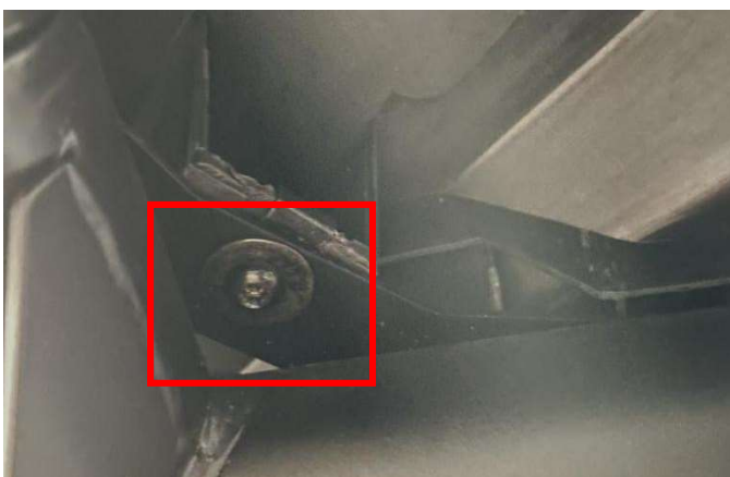
4. Finally, tighten the mounting buckles with screws. As shown in the picture:
