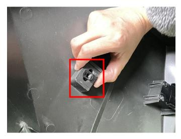
4. Attach the seal to the front of the roof (as shown)
