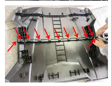
3. Use M5\*16 self-tapping screws to fix the iron brackets on the limit seats of the roof, and clamp the matching steel clips at the circled places as the picture shows:
